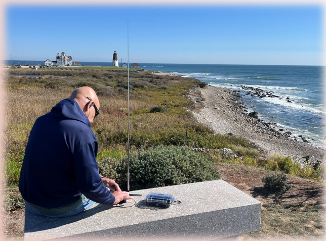
AJ1S Operating from Camp Cronin State Recreation Area US-10542 Pt. Judith RI - 10/20/2024 Elecraft KH1 with 4ft whip on 20m
